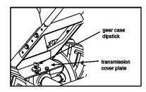
you add to the front transmission, you must wait a short period of time for the oil to follow rearward and equalize in both front and rear. The dipstick will read correctly on level ground for both gear units.
